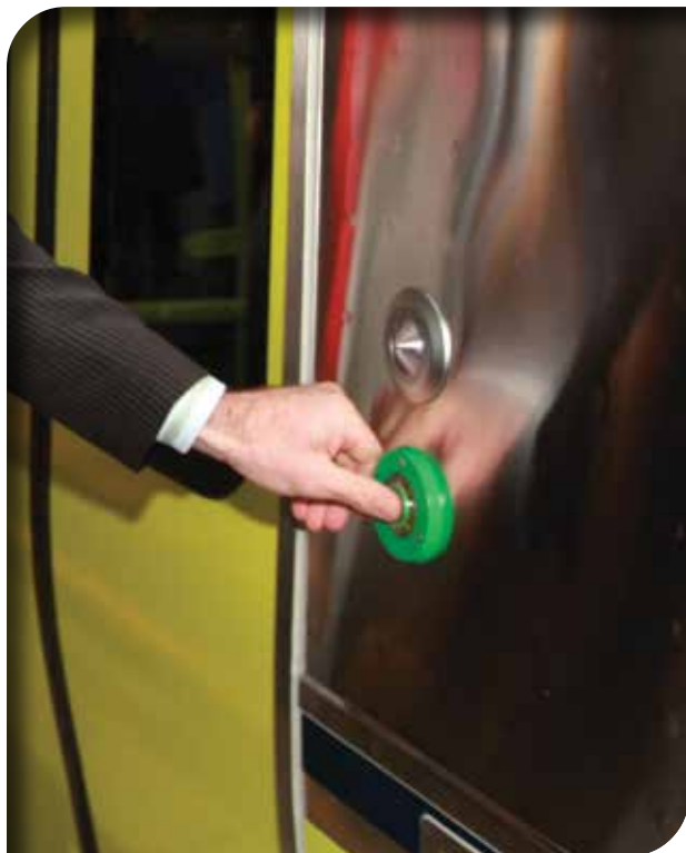
Audio warnings sound when the doors are automatically closing
