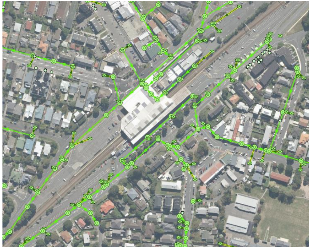
Figure 4 Existing Stormwater Network
