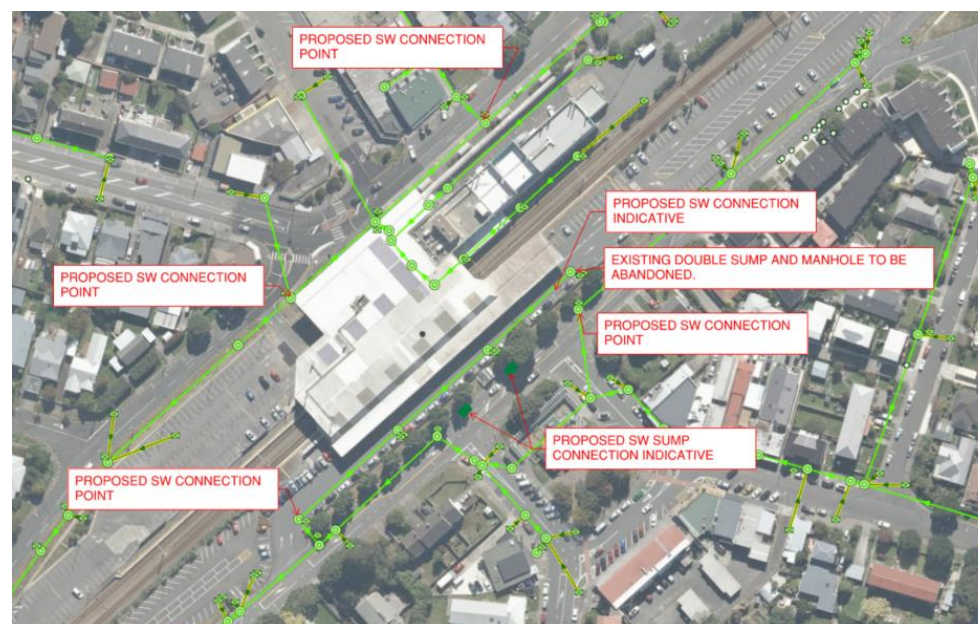
Figure 6 Stormwater Connection points (WWL GIS)
