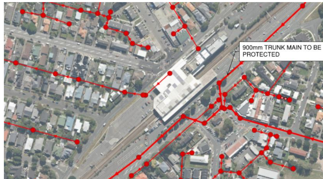
Figure 7 Existing Wastewater network (WWL GIS)
