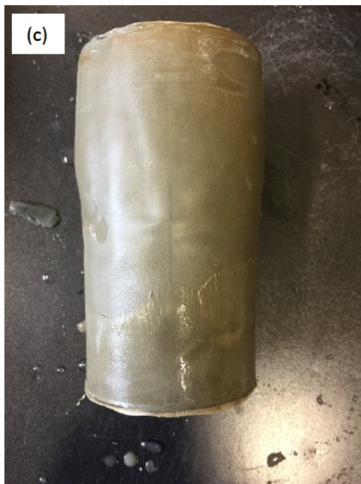
Figure 3: Condition of the specimen: (a) after undrained cyclic loading and before post-monotonic loading; (b) after post-monotonic loading; (c) after post-monotonic loading without the membrane.
