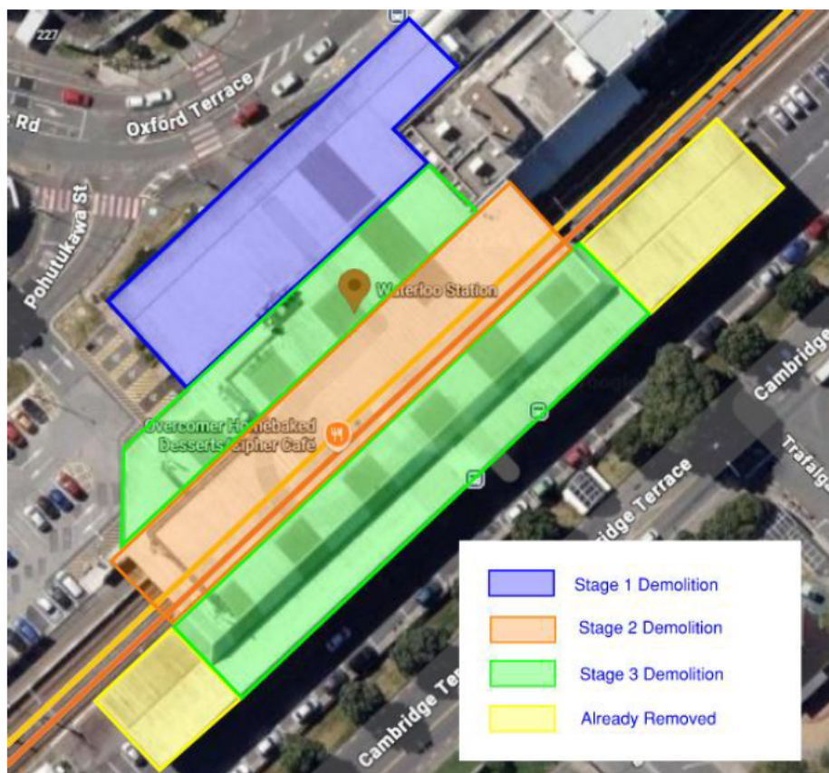
Figure 2 – Proposed Roof Structure demolition staging – Plan (NTS.)
