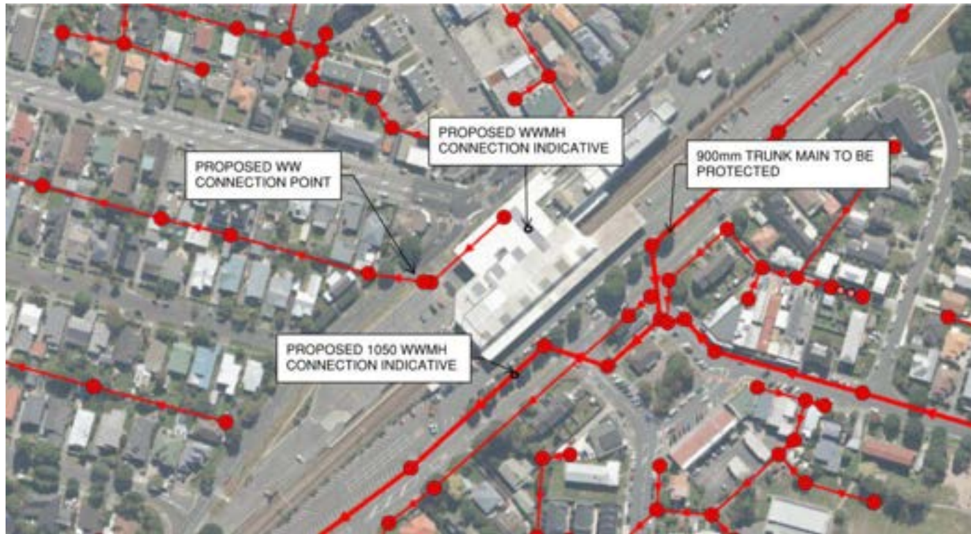
Figure 8 Proposed Wastewater connection points (WWL GIS)
