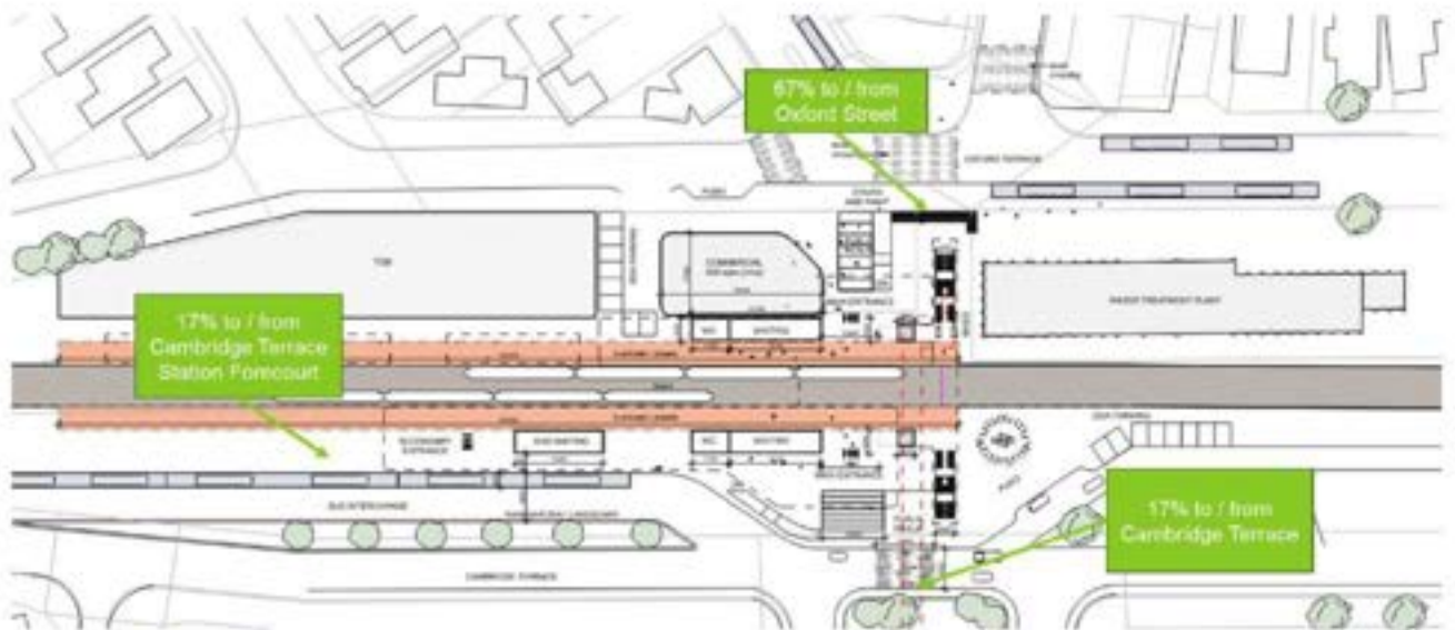
Figure 4-1 Waterloo Station assumed entrance splits
