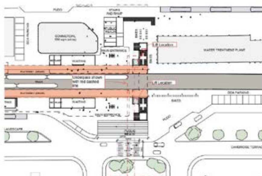
Snippet from Reference Design Drawing 1002 showing lift locations and clash with the underpass
