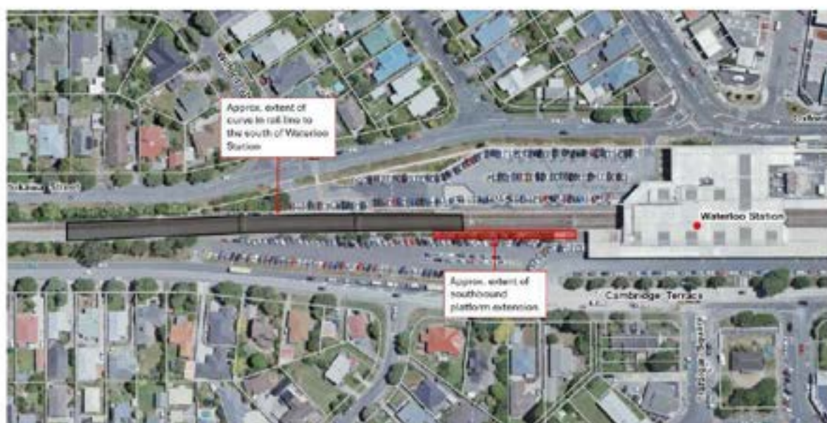
Figure: Aerial image taken from GWRC GIS, showing a markup with the location of the southbound platform extension and curve in the rail line to the south of Waterloo Station.
