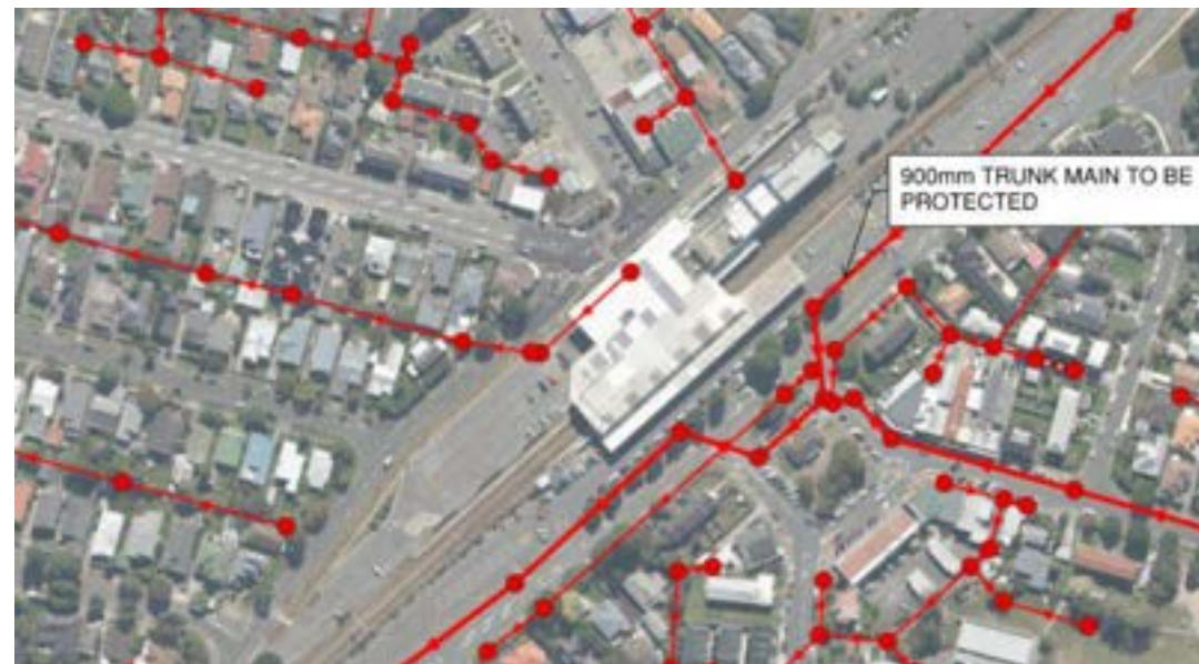
Figure 7 Existing Wastewater network (WWL GIS)
