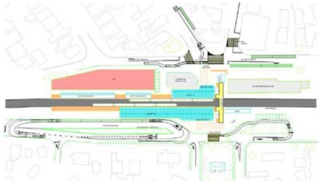
Figure 5-1: Vehicle tracking - bus interchange and PUDO
