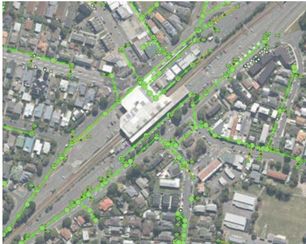
Figure 4 Existing Stormwater Network
