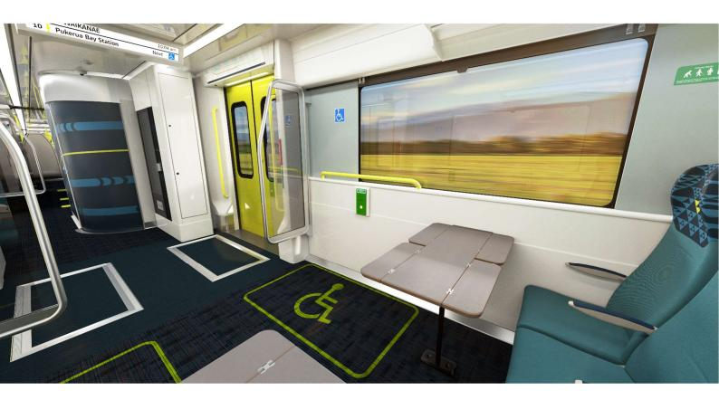
**Accessibility**. Each five-car Tūhono BEMU consists of two driving cab vehicles, and three intermediate vehicles. All intermediate vehicles have near level boarding access with a sliding step at each door for safe and accessible boarding.
